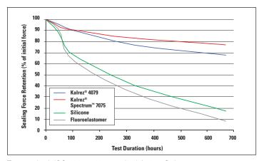
Test method: ISO 3384: 1991, method A, 214 O-ring
