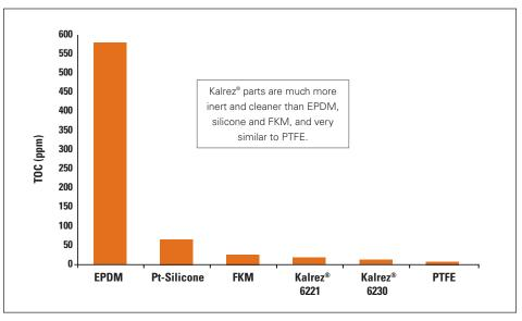
EPA method 415; TOC tests performed on 1" sanitary seals, immersed in 50 mL of sterile WFI at 100 °C/24 hrs. The solution was then diluted to 100 mL and analyzed.
