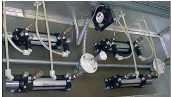
Pneumatic cylinder testing
