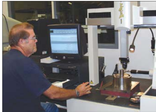
CMM: Coordinate measuring tool inspection
