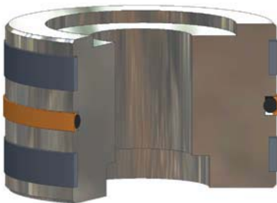
CP installed in Piston Gland
