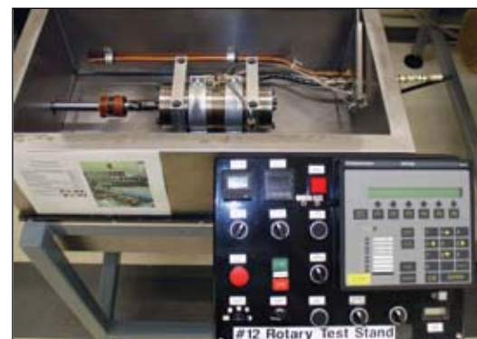
Rotary hydraulic testing
