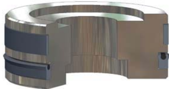
Type B PolyPak installed in Piston Gland
