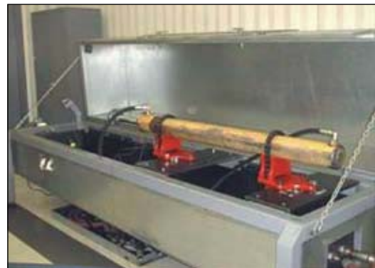
High pressure hydraulic leakage testing
