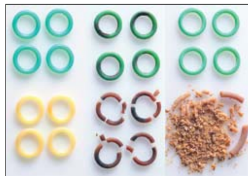
Figure 2-10. Progressive effect (hydrolysis) of high temperature water on standard urethane seals (yellow) vs. Parker Resilon WR (4301) seals (aqua).
