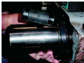
Installing the Seal
