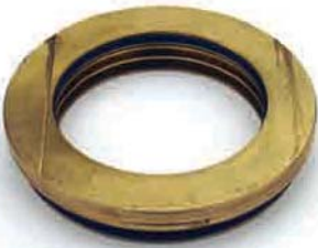
Failed Seal Resulting from Improper Installation
