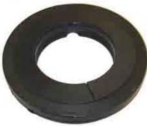
Failed Seal Resulting from Improper Fit
