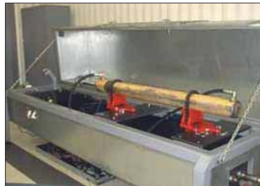
High pressure hydraulic leakage testing
